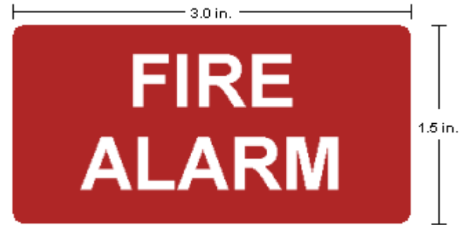
FIGURE M-2: Fire Alarm Exposed Conduit Label
